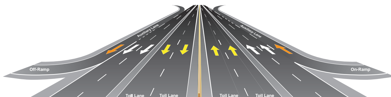
Proposed C-470 Ultimate - 2 Tolled Express Lanes in each direction plus 2 General Purpose Lanes in each direction with Auxiliary Lanes (select locations)
